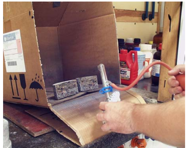
Figure 3.5 - Point-one M silver nitrate solution sprayed several times to the freshly split specimen [4].
