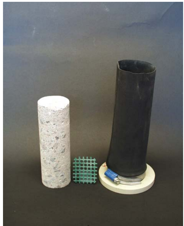
Figure 3.9 - Specimen in a rubber container, immersed in distilled water (internal frost resistance tests) or in a Sodium sulphate solution, 18 g/l distilled water [37], seawater from Barsebäck with 1% NaCl or distilled water (sulphate attack; performance in sea or fresh water).
