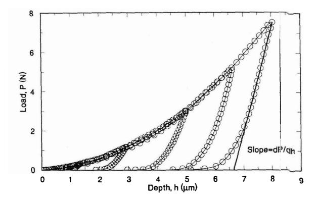
Figure 2: Load-depth plots at different maximum loads for sample EB4.
