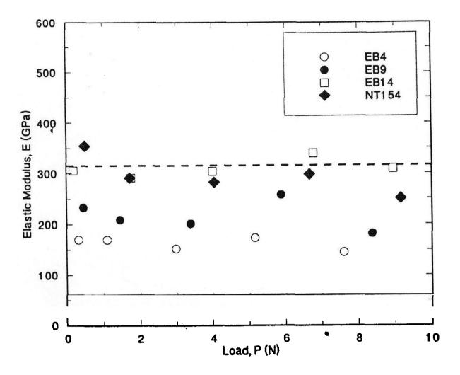
Figure 6: Elastic modulus vs. load calculated for four HIPed Si<sub>3</sub>N<sub>4</sub> materials using equation (4). Each point is the average of two readings. The dashed line represents E=315 GPa as provided by Norton/TRW for NT154.
