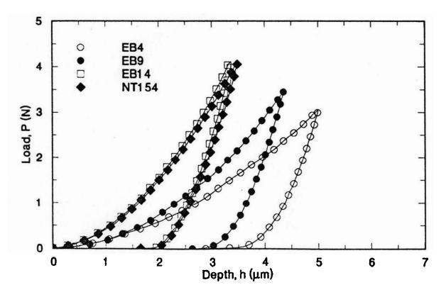
Figure 4: A comparison between load-depth plots obtained for samples EB4, EB9, EB14 and NT154 at the same total displacement.
